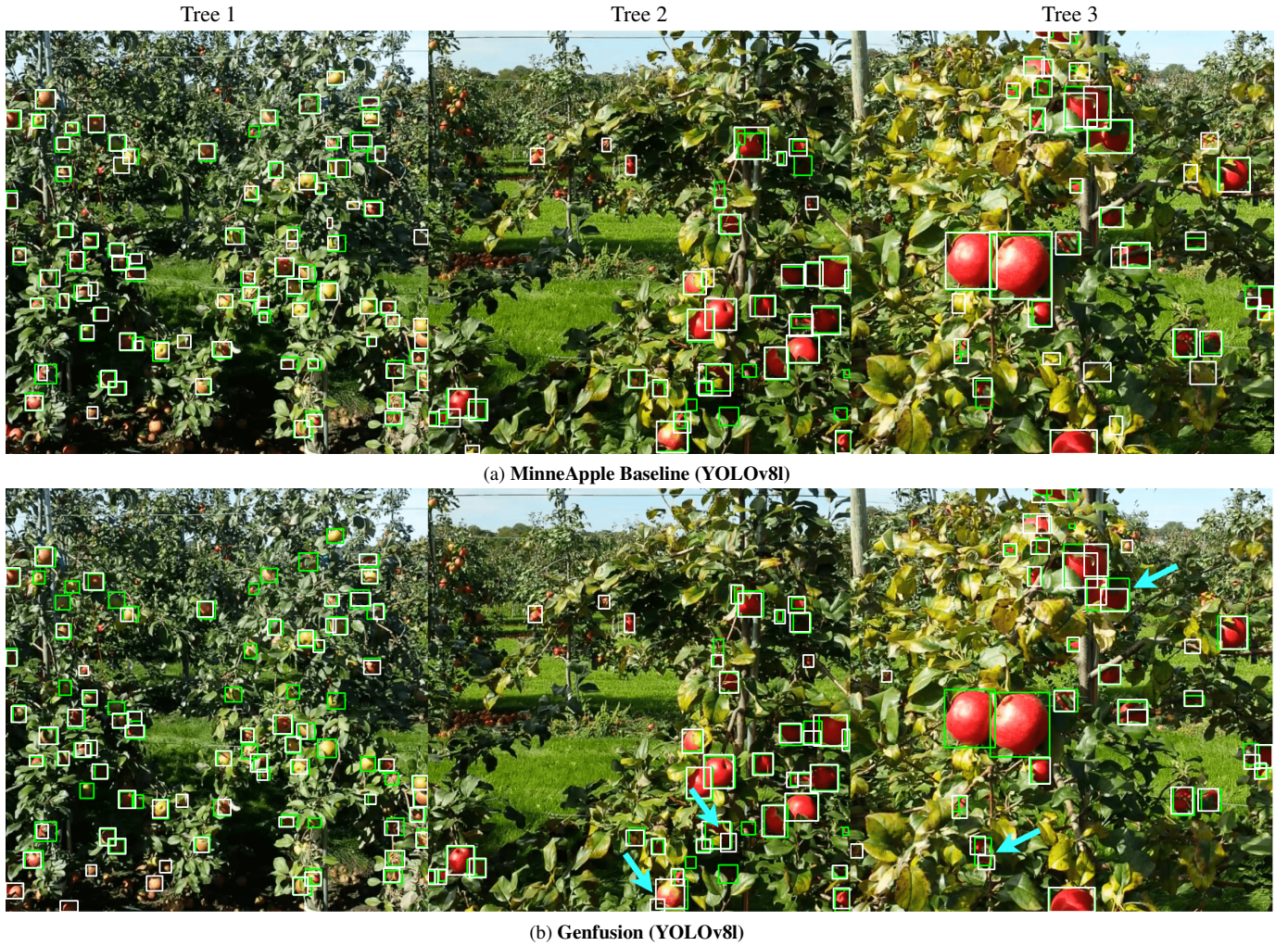
Fig. 5: The predicted (white) and ground truth (green) bounding boxes of the YOLOv8l Baseline and Genfusion model from three of the images from the MinneApple test set. The blue arrows indicate instances where the Genfusion model predicts two bounding boxes for a single apple.
